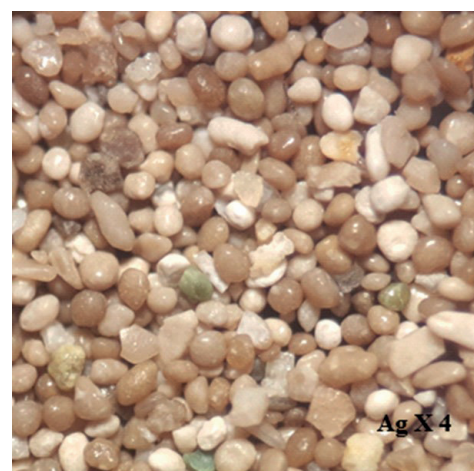
Fig. 11. Crushed and washed products on a binocular magnifier with the particle size fractions 0.53–0.100 mm of Bled El Hadba phosphate Rys. 11. Produkty rozdrobnione i umyte na lupie binokularnej o klasie ziarnowej 0,53–0,100 mm fosforanu Bled El Hadba
